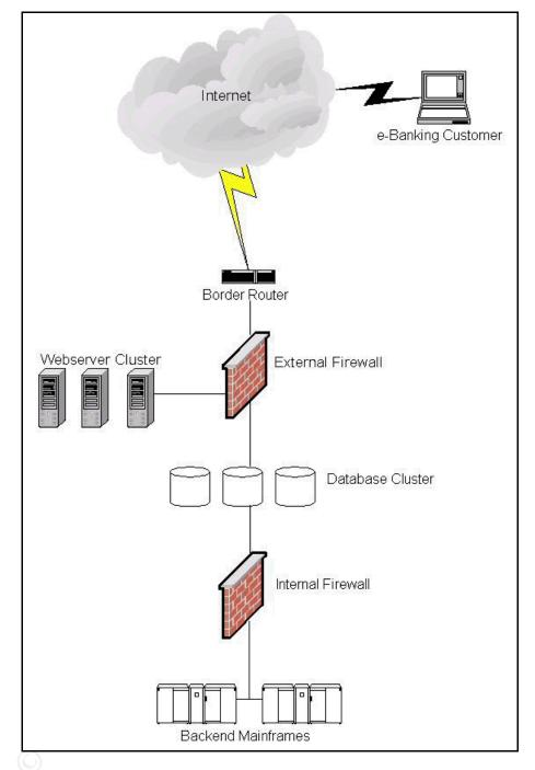
The External Firewall is dual-homed. One network interface connects to the web DMZ and the other connects to the internal network. The Internal Firewall provides further segmentation and protection of the Backend Mainframes. It does not directly connect to the network perimeter.
