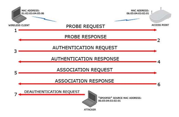
Figure 2.0: A deauthentication attack on an open wireless network
