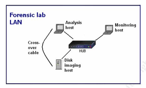
Physically and logically the lab LAN was isolated, or air-gapped, from any other systems. There were no physical (cable) connections from any of these devices to any other network or communications system. The lab LAN was setup in a low traffic, locked room and all systems were powered down when not actively involved in the analysis process.
