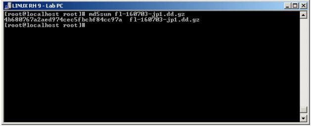
I extracted the DD image file from the fl-160703-jp1.dd.gz. Then, to safely work with the contents of the DD image, I mount it in read-only, non-execute mode as follows.
