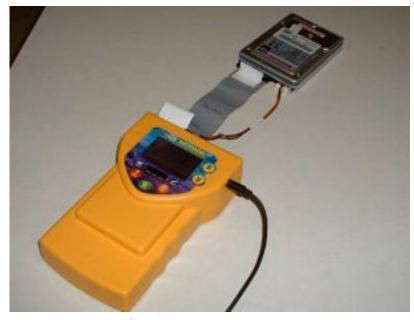
c. Be sure the SF-5000u recognizes the suspect drive and displays the expected number of sectors.
