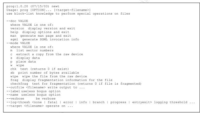
The output created by executing the downloaded version of Bmap yields almost identical results. The only differences are in the –mode option values. In the suspect version of the executable some of the mode options are abbreviated such as "m" instead of "map" and "c" instead of "carve" and so on. These minor cosmetic changes to the help listing could have easily been made at compile time.
