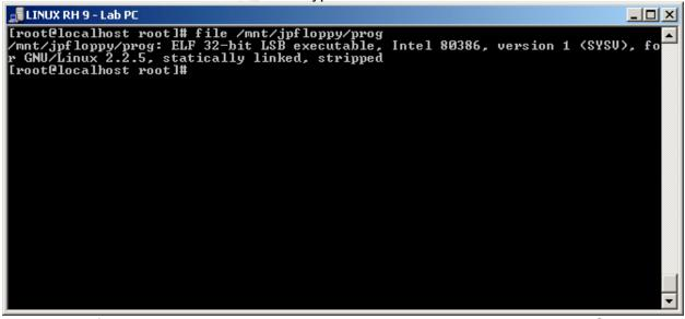
ELF stands for Executable and Linking Format, originally developed by Unix System Laboratories; it is an executable program file. We see from the FILE command output
