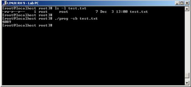
This would make sense because the Linux file system in use allocates sectors with 4096 bytes each.
