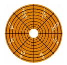
**sectors. gif** Here is another picture of a disk drive platter. This is the same platter, now one step higher, going from sectors to tracks and clusters.
