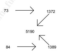
This packet also has TCP options set of opt 30. A series of packets are sent from MY.NET.208.226 port 1389 to 129.2.249.90 port 5190. These packets have all flags set except URGENT. The last packet of this type also has TCP options set of opt 30. The next packet in the sequence is from MY.NET.208.226 port 84 to 129.2.249.90 port 1389. A few seconds later the last packet is sent from MY.NET.208.226 port 1389 to 129.2.249.90 port 5190. For these last two packets all flags except URGENT are set.
