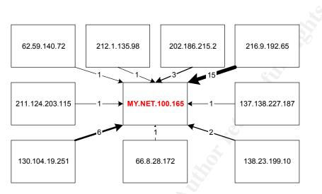
As we see from the link graph, two IP addresses were the responsible for sending most of the packets. And in the following link graph, it is possible to see the analysis of the combination of source and destination port numbers.
