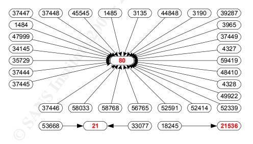
The target of most of these packets was port 80 while port 21 was hit twice. Port 21536 is an interesting one as scans from port 18245 to port 21536 have already been seen around on the internet.
