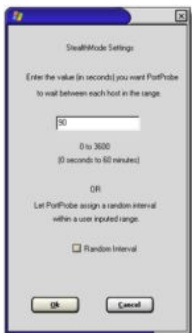
Fig. 1-15 In StealthMode, there is an option for a "static" timeout interval between probing multiple hosts, or there is an option for a newly generated random interval between each host.
