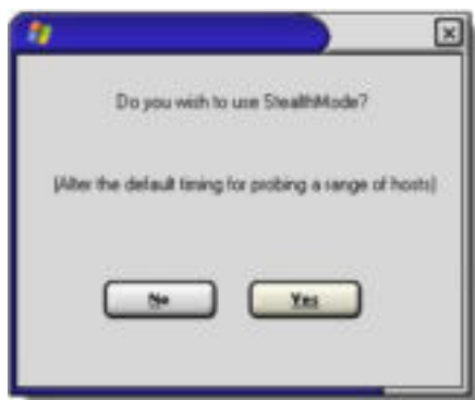
Fig. 1-14 When you are scanning a range, we have an additional option. The use of "StealthMode" is basically a random interval between probing each host to try to hide the probes.
