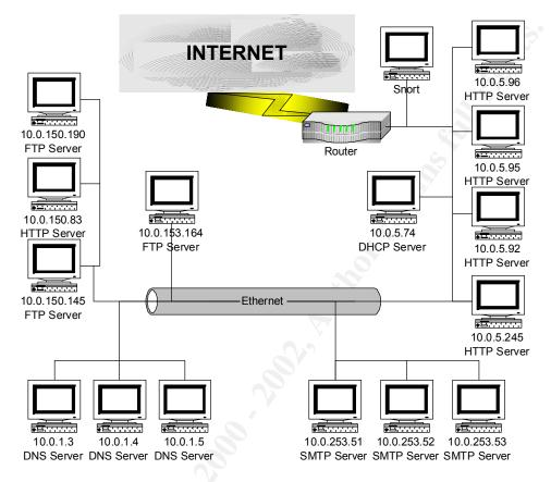
This is the assumed topology of the GIAC University Network. All assumptions here were based on traffic that was seen in the supplied Alert, Scan, and OOS data files. If there are services that I have represented here which are actually not running on these servers than further investigation is necessary.
