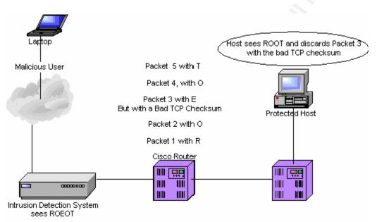
This is another Insertion Mechanism similar to the TTL Expiration but Packet 3 is sent with a Bad TCP Checksum. Since the Intrusion Detection System does not verify the TCP checksum of every packet, this can be successfully used to evade the detect. The Protected Host at the other end discards the packet with the bad checksum and sees ROOT.
