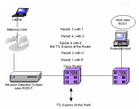
In this example the Malicious User sends 5 packets to send ROOT to the remote host with Packet 3 being the crafted packet whose TTL expires at the Cisco Router thus the Intrusion Detection System sees **ROEOT** while the protected host sees ROOT.
