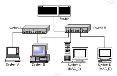
In the above diagram, assuming System C sent a packet to System D and the MAC address of System C and D is MAC\_C and MAC\_D respectively. Below is a simplified example showing how a switch can "learn" about traffic:
