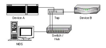
When using either a hub or switch for this purpose, be certain to consider those bandwidth issues mentioned previously. High load will cause packet loss which will affect the performance of NIDS.
