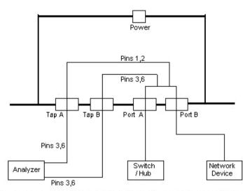
UTP Tap IL/1 passes in-line power per "IEEE 802.3af DTE Power via MDI" specification.
