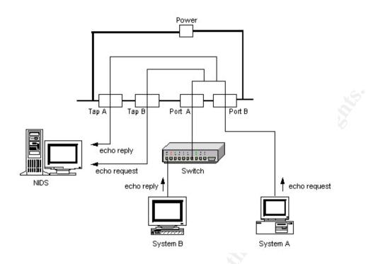
Using the above diagram as the setup, System A does a "ping" to System B. Below shows what the tap capture when an NIDS is connected to either of the tap.
