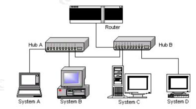
Systems connected together using only hub(s) are under the same collision domain. In a collision domain, only one system is allowed to transmit traffic at an exact instant of time [3]. If two systems in the same collision domain transmit at an exact instant of
