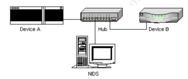
In the diagram, a hub had been introduced into a link whereby the traffic needs to be monitored. Device A and B can be a router, switch or server. The NIDS will be able to see the traffic passing between Device A and B due to the broadcast property of the hub.
