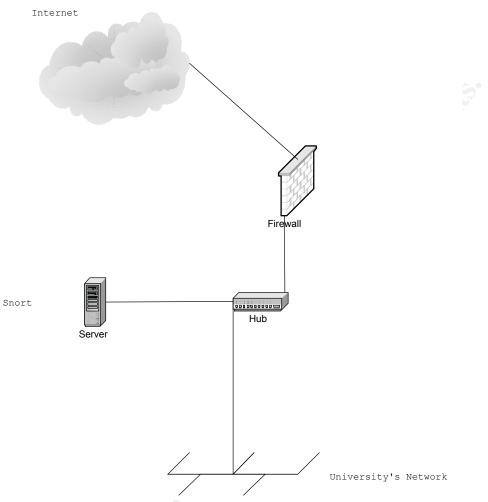
I propose that the IDS infrastructure be upgraded to encompass at least two sensors, one outside the firewall and one inside the firewall. Having these two log to a central database and using a web based front end would enable the system admin a much easier time of sorting trough the alerts. A diagram of the improved IDS infrastructure would also look like the following graphic.
