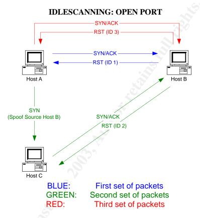
We have now covered most of the concepts in the above diagram. Don't let the diagram appear more complicated than it is. We'll go through the process step by step to see how we can make idlescanning work for us. Continue to assume that Host A is the attacker in this example. This example also assumes that Host B uses incremental IP ID's and is not actively communicating with other hosts on the network.
