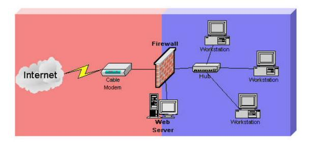
On my home network, a Cable Modem provides uplink to the service provider. Behind the cable modem is a Linux Firewall running IPTables. The Firewall has three NICs, one that connects to the outside world, one for the internal network and one to connect to the web server.
