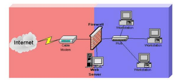
On my home network, a Cable Modem provides uplink to the service provider. Behind the cable modem is a Linux Firewall running IPTables. The Firewall has three NICs, one that connects to the outside world, one for the internal network and one to connect to the web server.
