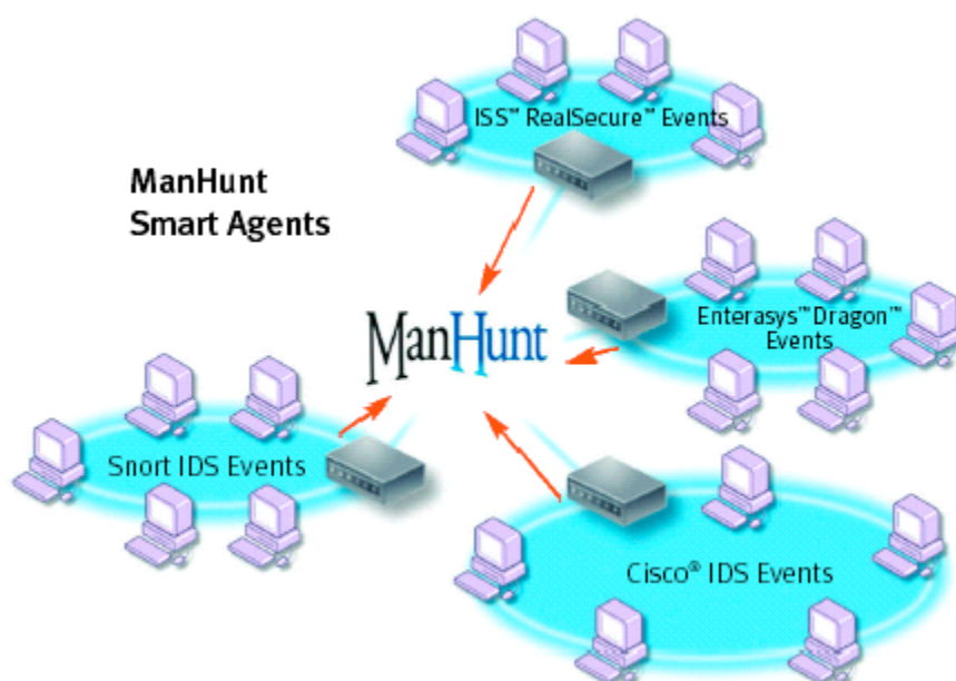
Figure 2: ManHunt integrates with Third-Party Intrusion Detection Systems to provide Enterprise-Wide Event Correlation and Analysis. [2]
