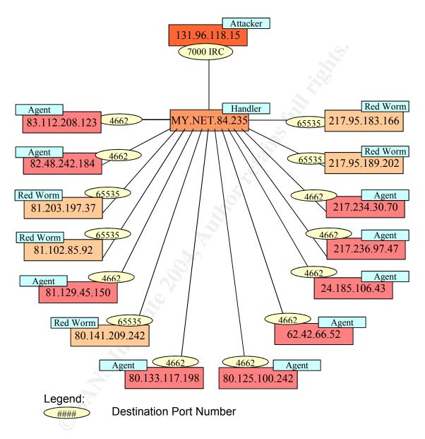
This link graph shows the relationship between the Attacker, Handler and Agents of mstream DDOS (Distributed Denial of Service) attacking system. Only the Handler is sitting inside the University's network. Five other systems were RedWorm infected and were connected to the Handler.
