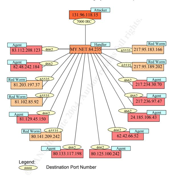
This link graph shows the relationship between the Attacker, Handler and Agents of mstream DDOS (Distributed Denial of Service) attacking system. Only the Handler is sitting inside the University's network. Five other systems were RedWorm infected and were connected to the Handler.
