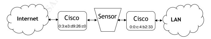
It is possible that a firewall on the monitored segment (LAN) side is present or asymmetric routing is being used (egress traffic is routed differently than ingress). The reasoning for these conclusions will be explained in more detail further within the analysis of the detect.
