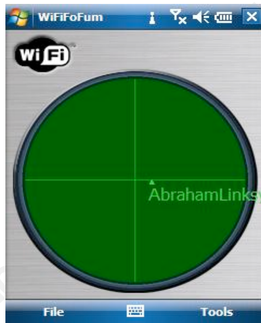
Rogue AP detection using WiFiFoFum
