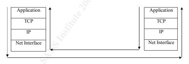
If you look at a TCP data thru a sniffer you will notice that the header on a typical IP datagram is 20 bytes. TCP has no idea what the contents of the bytes are. Each TCP segement contains the source and destination port number to help identify the application that is doing the communicaitng. The contents of the bytes are left up to the application to read and interpret.
