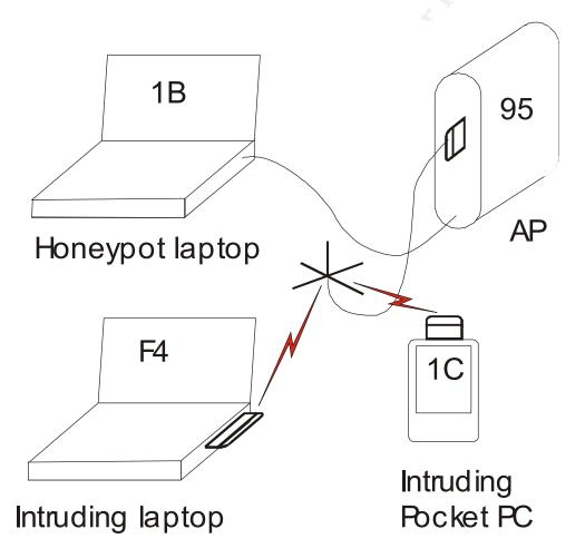
Here a laptop running conventional sniffer software, in this case CommView<sup>11</sup>. The laptop and AP are connected with an Ethernet cable and the AP is connected to a 2.4 Gigahertz antenna. The antenna used in this case is a simple vertical quarter wavelength
