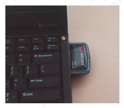
**Typical wireless LAN card in a laptop** – the only equipment that an intruder needs to connect to an unprotected network access point. Sniffers, scanners and protocol analyzers may also be used to conduct various attacks with this setup. <sup>2</sup>
