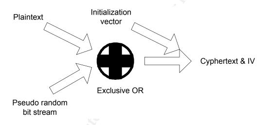
After the exclusive-or the initialization vector (IV) is appended to the cyphertext so it is available at the receiver for reversing this process. When the 802.11 standard was written a weakness in this process was recognized.
