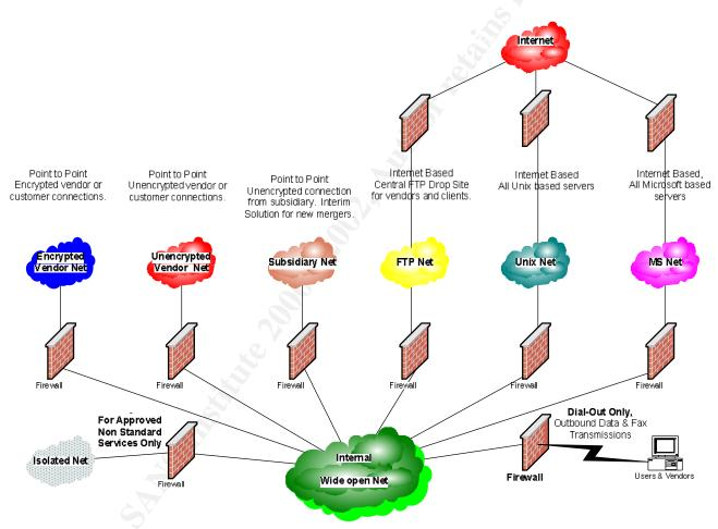
The Wide Open Net is by far the largest segment of our network, with most user machines sitting inside it. The other nets have connections from the Wide Open through firewalls with strict ACL's on their way out to the Internet, and the Internet Based Firewalls contain our IDS system on the perimeter. We run our Host Based IDS system in the Wide Open net area, protecting servers in the other nets with a specific business need.
