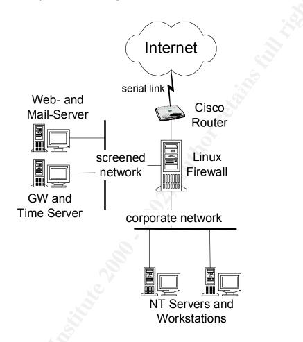
This is a example network of a company, called Company X. It is a small to medium network as shown above. This is a replication network of one of our customer.
