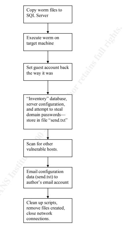
Note that the automated attack is very linear—it only really uses one major decision point in its logic. If a step doesn't work, the attack moves on to the next step. The only thing which causes a complete abort is if the target machine is protected. The attack is not guaranteed to succeed, though. Even if it locates a
