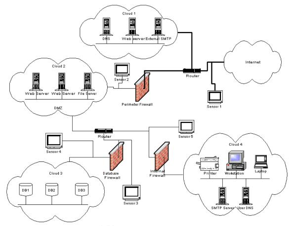
Our network has one main feed to the Internet. That Internet feed comes directly into our Cisco 6509 router. That router was running Cisco IOS version 12.01 at the time Nimda struck. That router separates the traffic between what is directed at three servers considered to be on our 'dirty' feed and our firewall that leads to a DMZ and then on into our network. By 'dirty' we mean not protected by any firewall and those lines are shown in the above diagram as being in bold.
