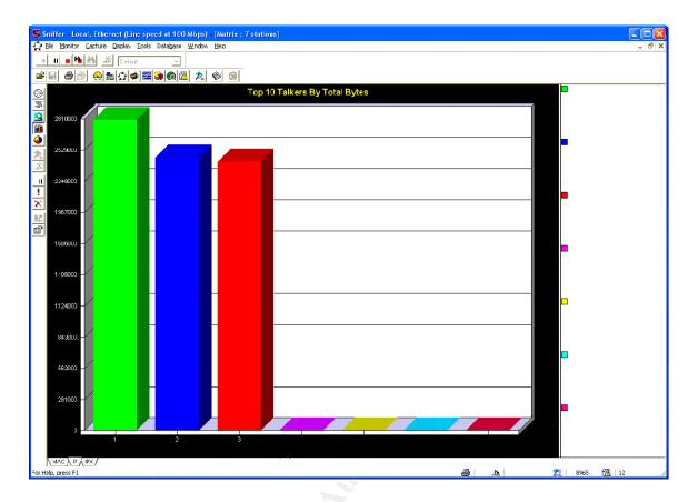
After only 30 minutes or so of running the Sniffer network analyzer program, it shows the 3 foreign hosts connected to the server as being the top talkers by a wide margin. Again, the IP addresses have been removed.
