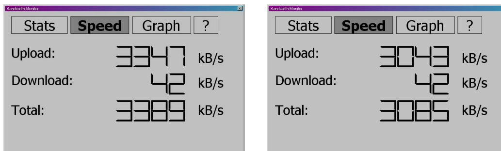
Figure 5. Bandwidth Monitor showing used bandwidth (kilobytes/sec) on both SQL Slammer infected machines (Bandwidth Monitor Program, courtesy of http://www.idyle.com )
