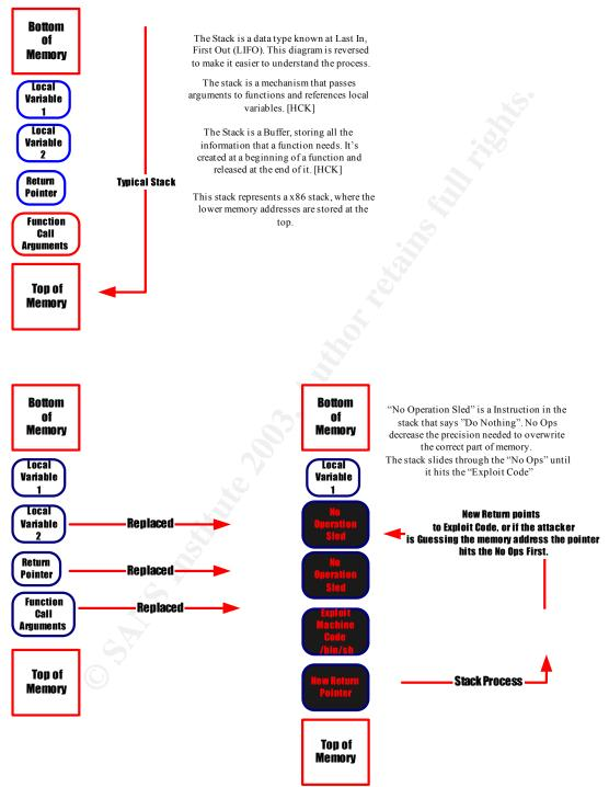
Here we see the attacker over writing the lower memory addresses [top of memory], having the return pointer over write higher memory addresses [bottom of memory].
