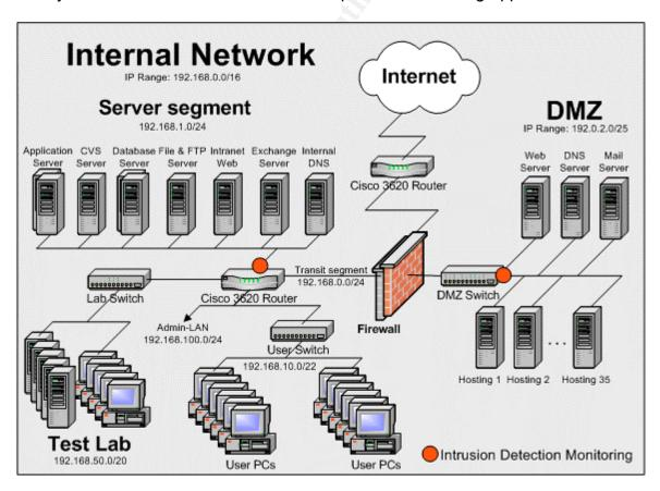
Internet access is established via a 10 MBit leased line with a Cisco 3600 router handling the traffic. There are some basic anti-spoofing egress rules in place on that router:
