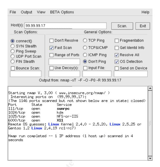
The following screen capture is of nmap scanning the intrusion detection system for open UDP ports. The number of ports left open tell the technician that more security measures are needed.
