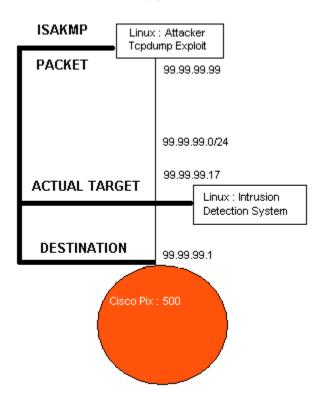
The attacker using a packet manipulating program sends a malformed ISAKMP packet to the Pix firewall. The intent is for the intrusion detection system running tcpdump versions 3.6 - 3.7.1 is to cause an infinite loop. Other types of packets such as NFS, BGP, and RADIUS are able to cause an DoS attack as well. The tcpdump exploit program is compiled and executed with the destination IP address 99.99.99.1.
