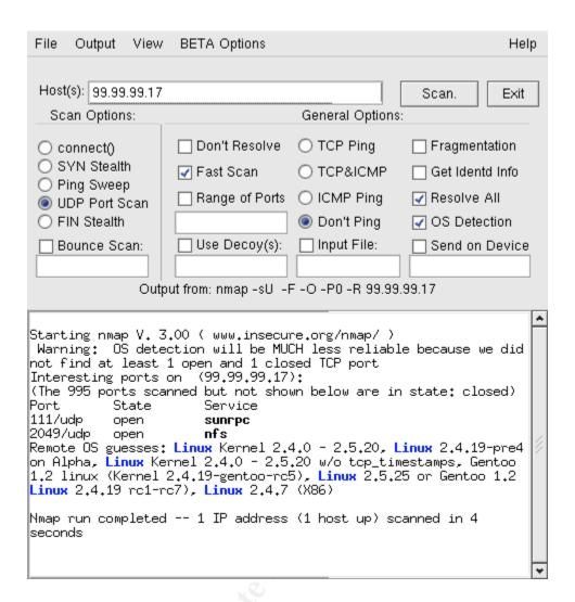
The following screen capture is of the nmap scanning the Pix for open ports that may be used for setting up back doors. The Pix has better security applied than the intrusion detection system at this time.
