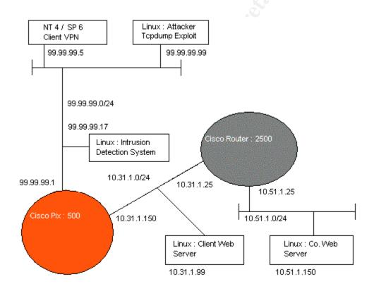
The Windows NT box represents clients that access the network using a secured network via IPSEC and non-secure access to the web server as well. NT version 4 is installed with service pack 6. Cisco VPN client 1.1 is used to connect to the Pix via IPSEC tunnel. The SafeNet - Cisco Secure VPN Client version 1.1 is setup with the following parameters:
