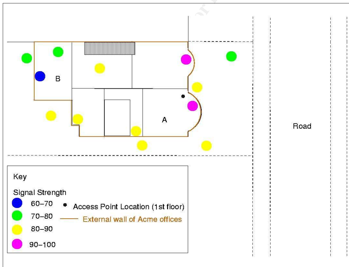
Figure 38: AP signal strength inside and just outside Acme offices.
