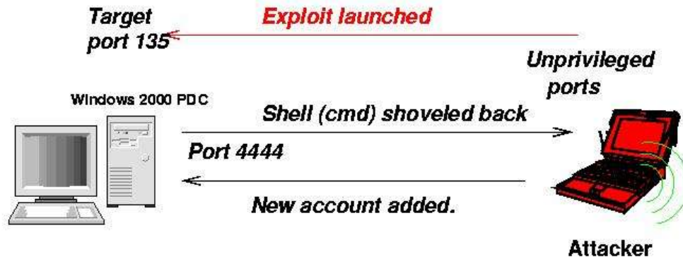
Figure 15: Breakdown of attack and subsequent actions.
