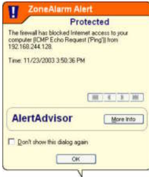
Figure 7 – ZoneAlarm Alert – Ping From Infected Host [17]
