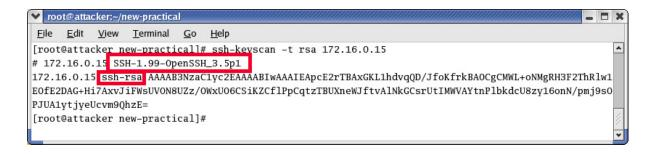
In the above graphic, the output was not redirected to a file, but instead captured in the screen shot. The above results shows that the server is running version 3.4p1 of OpenSSH. It also indicates that the version 2 option for rsa keys (ssh-rsa) is supported. (Version 1 keys for rsa format are designated with rsa; version 2 keys are designated as either ssh-rsa or ssh-dsa.)<sup>17</sup> Due to the mathematics involved, rsa keys are faster to generate than dsa keys.
