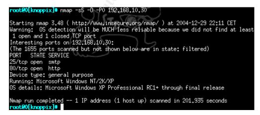
Showing that the *http* and *smtp* ports are open, the remaining ones are filtered by the firewall.
