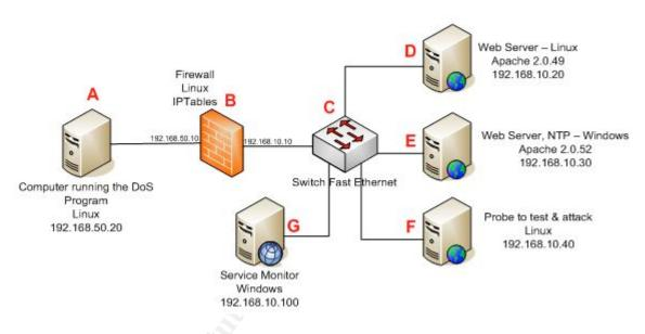
To deploy this laboratory a minimum of six computers are needed and one of them needs two network interfaces (to work as firewall).
