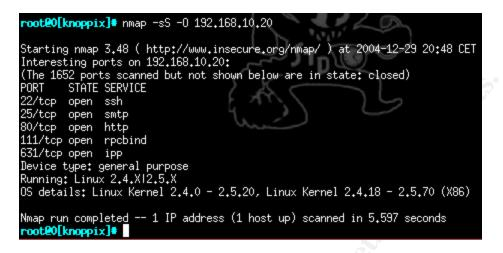
Showing that the *ssh*, *smtp*,*http*, *rpcbind* and *ipp* ports are opened.
