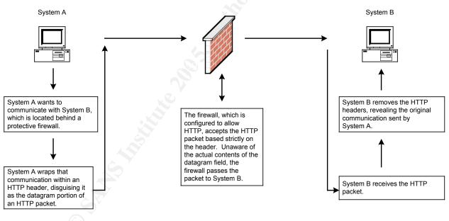
The following diagram illustrates the basic concept of HTTP tunneling:
