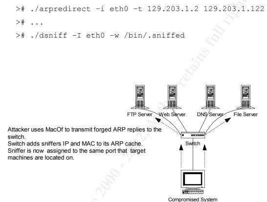
Now all traffic directed towards the target machine will be transmitted on the same port on the switch as the sniffer.
