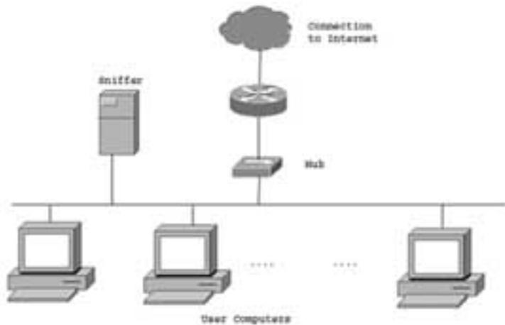
**Figure 4. Net configuration of the commercial offices**
