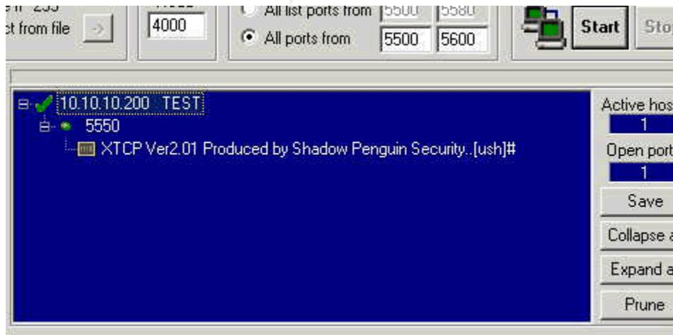
You will be able to see the shell prompt "[ush]#" exactly like in Unix, when you are connected to the target:
