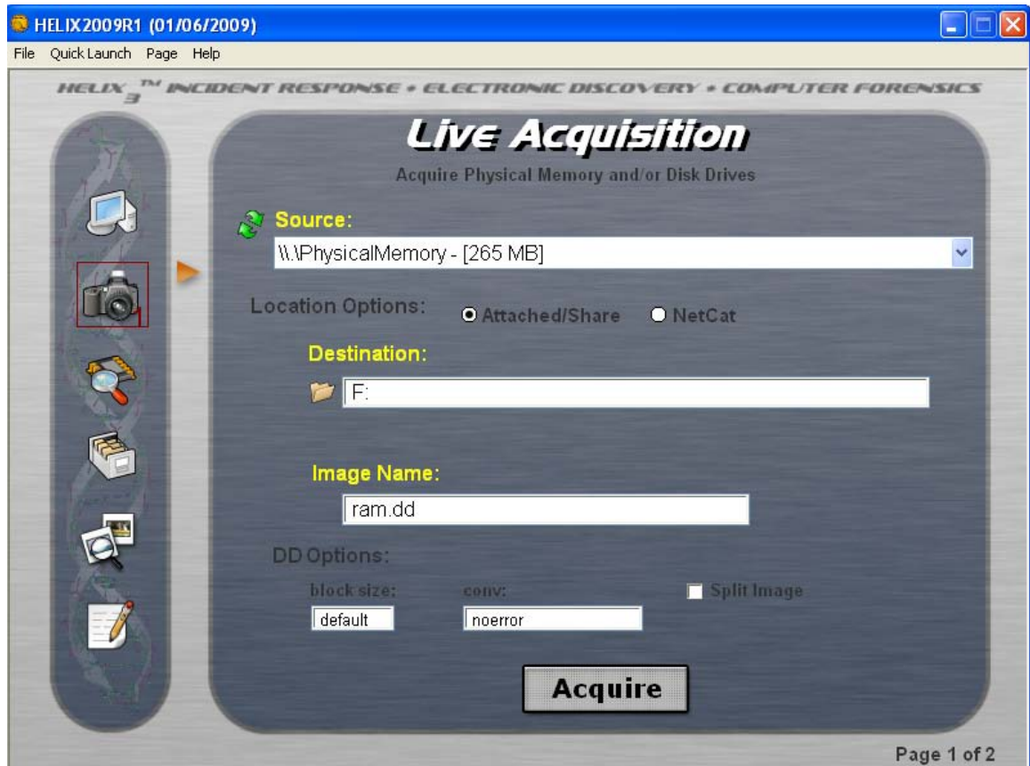
Figure 14: RAM Acquisition with Helix
