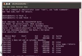
A list for each device on the system will appear as in the screen shown on the left. For each physical drive that needs to
