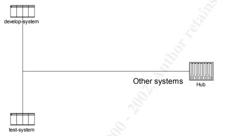
This drawing represents the physical connections involved in the local configuration. The connections between the two systems shown and the hub use a 10 MHz Ethernet cable. The reason for this is because the rest of the connections at this location use 100 MHz Ethernets. The hub also serves as the gateway to translate from 10 MHz to 100 MHz. (HP's PA-RISC hardware of the vintage in use only supports 10 MHz.)
