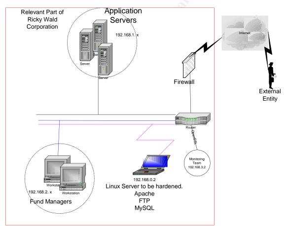
Below is a high level diagram of the relevant part of the network
