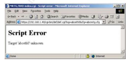
Since the def.cgi script is hard-coded to only open the defmrtg.cfg file, the abceth0 MRTG target is not found and so the message above is displayed. To ensure that the syntax is correct, the url is modified to read: <a href="https://192.168.1.40/cgi-bin/abc/abc.cgi?log=abceth0&cfg=abcmrtg.cfg">https://192.168.1.40/cgi-bin/abc/abc.cgi?log=abceth0&cfg=abcmrtg.cfg</a>. The following screen is displayed after logging in as the abc user:
