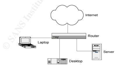
The network is connected via a HUB/Router. All the machines on the internal network have a private ip-address and only the services required from the outside network are
