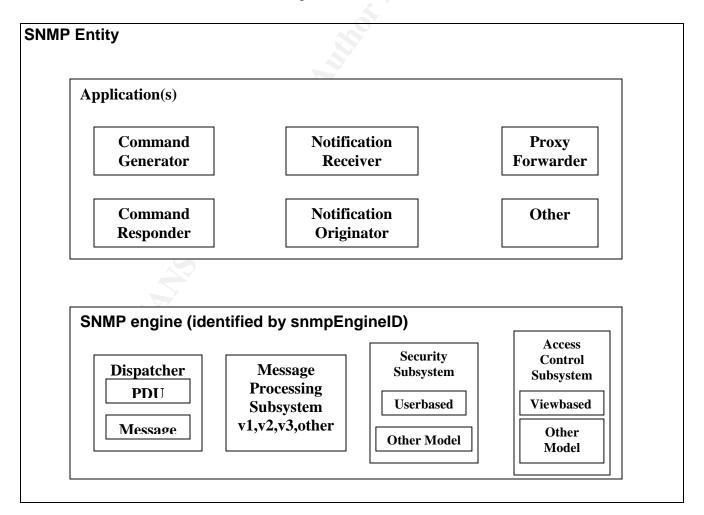
SNMPv3 is a much more complex system than the two previous versions. It involves taking the original SNMP engine and adding the security and access control sub systems.
