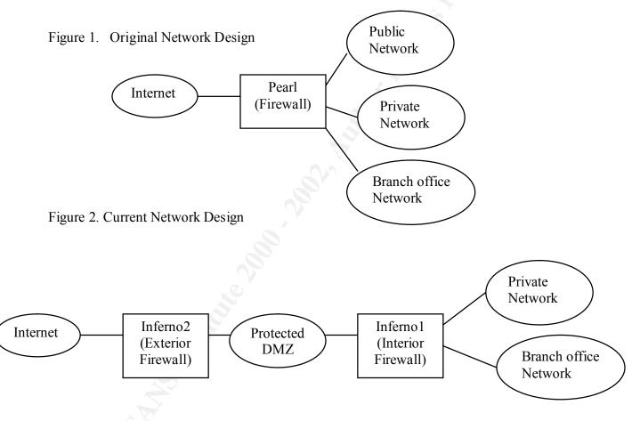
This perimeter defense design is superior because it allowed different firewalls with different responsibilities. The exterior firewall (Inferno2) protects the Internet servers on the DMZ from general access from the Internet as well as defense in-depth for the second interior firewall (Inferno1) which protects the private network with a more stringent ruleset as well as acting as a NAT gateway to the Internet
