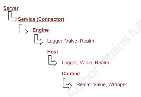
It is useful to understand how a "hit" traverses through the nested Tomcat components. The diagram below illustrates this. For this example, we will use:
