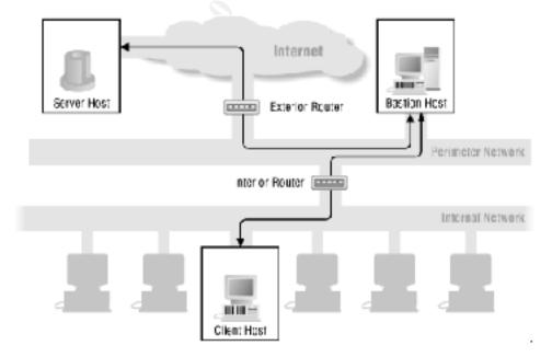
GIAC Enterprises has set up their network to use two packet-filtering routers:
