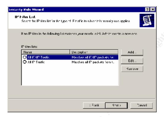
To create a new IP filter, click Add. For example, if you had a DMZ web server you could write a rule that allowed only HTTP and HTTPS traffic by blocking all ports except 80 and 443 respectively and thus allowing ICMP packets to pass.
