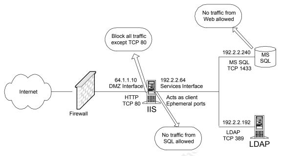
As practice, what additional IPSec rules are necessary to only permit TCP 389 from web server to LDAP server? The LDAP server is single homed and has the IP Address of 192.2.2.192. Remember to create a flexible rule that would work even if additional LDAP or web servers were added at a later date (Hint: review the Network Information table). The answer is in Appendix A.
