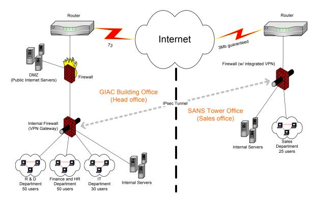
GIAC choose to have a VPN network to connect both offices, all inter-office communication including file sharing and E-mail will be encrypted by the IPSec tunnel between the two firewalls, so any potentially sensitive inter-office communication travelling on the Internet are secured.
